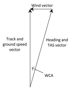
This MDR technique works for the relatively small WCAs which are typical for medium to high TAS values (the ground speed (GS) therefore can be assumed to be equal to the TAS for application of the 1:60 rule).
