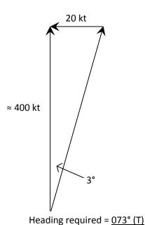
GS is determined by using the headwind/tailwind example previously explained.
